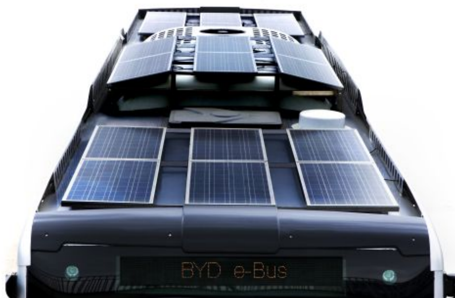
Figure 16: Solar panel on the roof used for the air-conditioning system [25]
