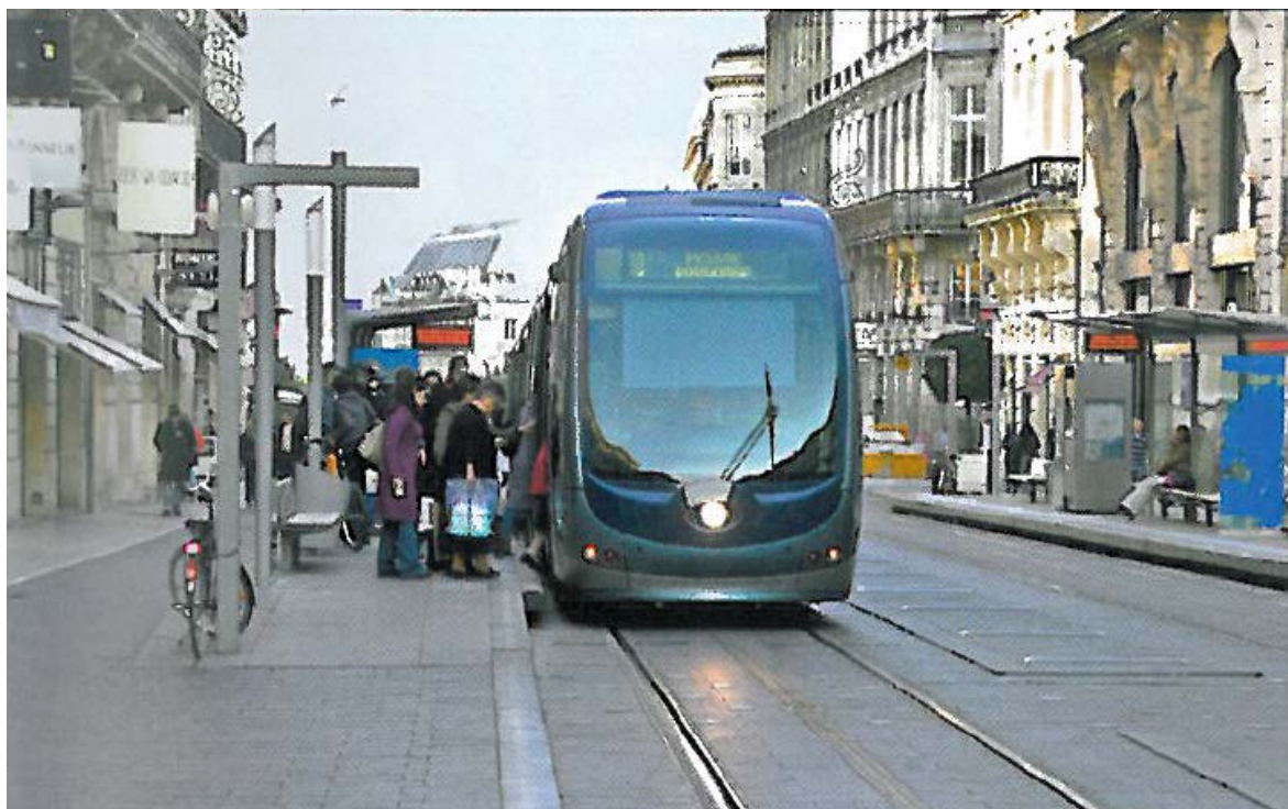
Figure 5: Power rail in the middle of the track in Bordeaux, France [82]
