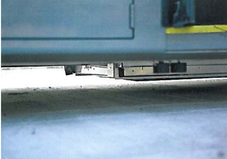
Figure 10: Vehicle components (secondary coil and antenna for segment activation) for energy transfer are mounted below the bus [101]
